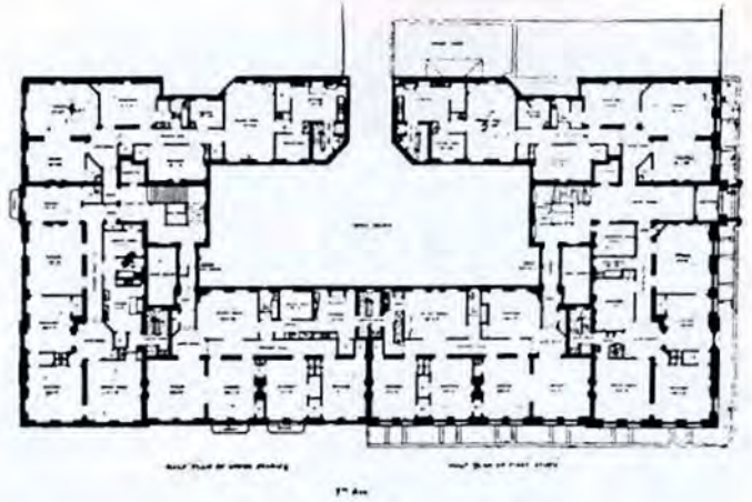
Fig. 22. Vancorlear. Henry J. Hardenbergh. 1879. Combined plan of first floor (right) and typical upper floor (left).
